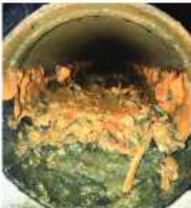
Dry Pipe Systems Trap Water
