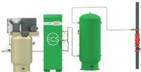
Wet Pipe Nitrogen Inerting Equipment Configuration
