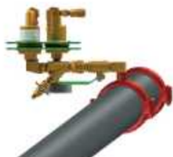
Air Vent Installation (Remote High Point)
